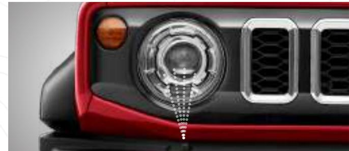
**MANUAL LEVELING LED PROJECTOR HEADLAMP WITH WASHER**
